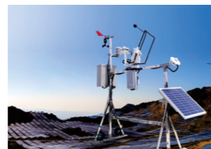
Photovoltaic environmental monitoring instrument
